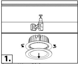
Cut out a 205mm Ø hole in the ceiling
