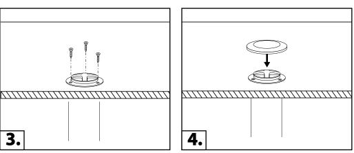
Screw in the light using the included screws.
