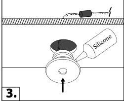
Apply marine grade silicone on the light or in the hole, then insert the light.
