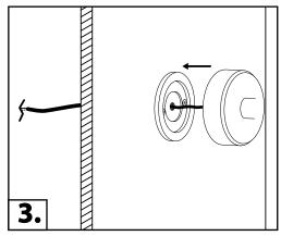
Route the cable through the hole and connect according to the electrical diagram.
