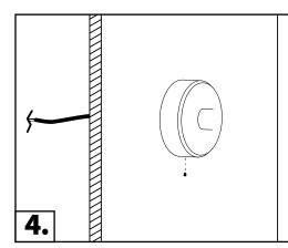
Place the light on the mounting bracket and screw in the included pinion screw to finish installation.
