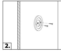
Screw in the mounting bracket around the hole with the included screws.
