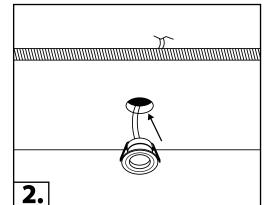
3. Press the spring clips backwards and insert the light into the hole.
