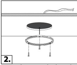
Screw in the mounting bracket, making sure that the countersunk screw holes are facing you, with the inluded screws.
