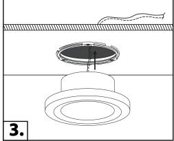
Route the cables through the hole and connect according to the electrical diagram
