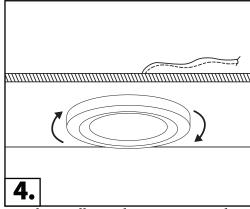
Finish installation by screwing in the light onto the mounting bracket.
