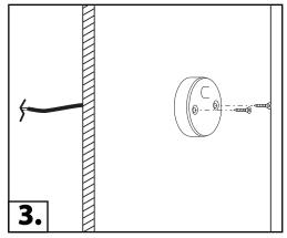
Screw in the light using the included screws.
