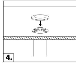
Install the cover plate back on to finish installation.
