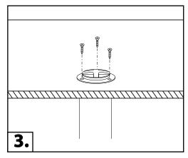
Screw in the light using the included screws.
