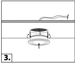
3. Press the springs backwards and insert the light into the hole.
