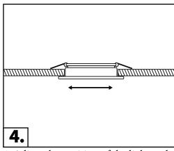
4. Adjust the position of the light and make sure it is well locked to finish installation.
