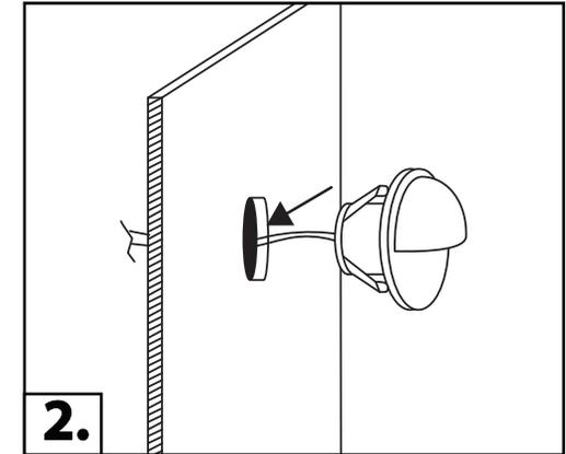
Route the cables from the light through the hole and connect the light according to the electrical diagram.
