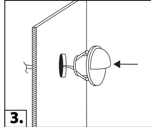
Push the light into the hole to so that the springs engage to finish installation.
