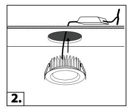
3. Press back the springs and insert the light into the hole.
