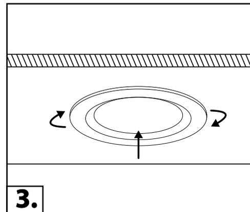
3. Screw the front back on again to finish installation.
