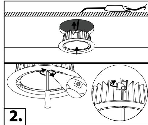
2. Connect the light to electricity according to the electrical diagram and install the light.
