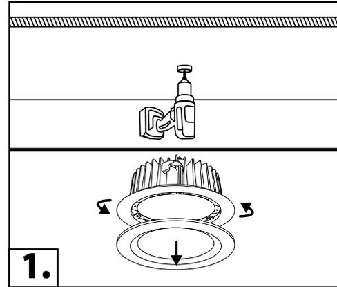
1. Cut out a 205mm Ø hole in the ceiling
