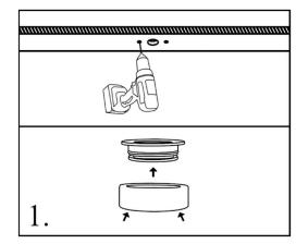
**2.** Screw in the base to the celling with the included screws
