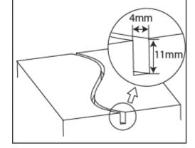
2. Gently push the LED Neon flex down in the cut mark.
