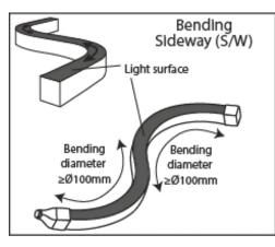
Do not pull or twist the LED flexible strip.
