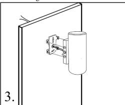
**2.** Screw in the bracket using two screws.
